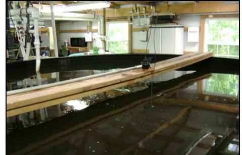
Boom over tank, from which remote camera is suspended
